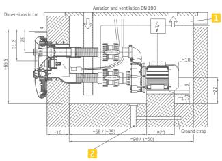
Sufficiently dimensioned drain required
